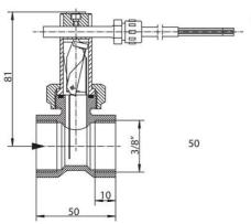
UR1 - loosen bolts, push the switching current tube into the desired position. Retighten the bolts. Normally closed (n.c.) or normally open (n.o.) as per table "Technical data"
